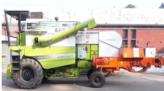
view of the developed baling attachment with self-propelled combine harvester
