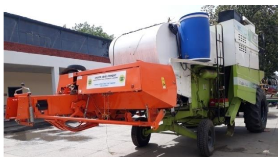
view of baling attachment with self-propelled combine harvester
