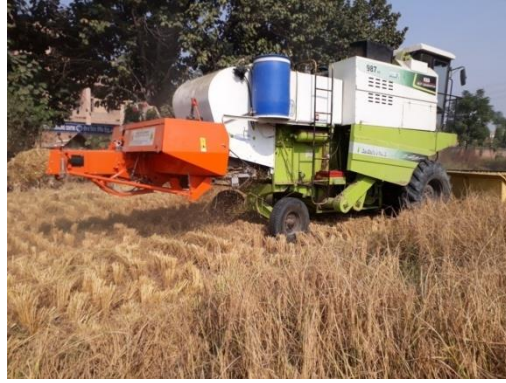
Bale ejected from the baling attachment with self-propelled combine harvester
