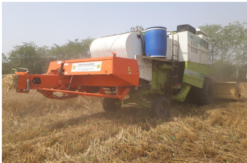
Combine harvester with baling attachment during the wheat harvesting
