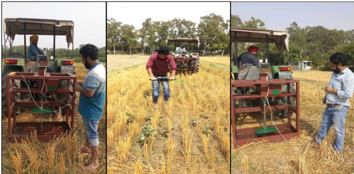
Fig. 3: Validation of the developed dual soil sensor system in the field under different treatments.
